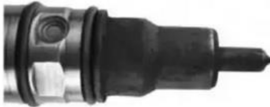
Figure 1: Lack of Copper Washer or Inadequate Torque Injector
